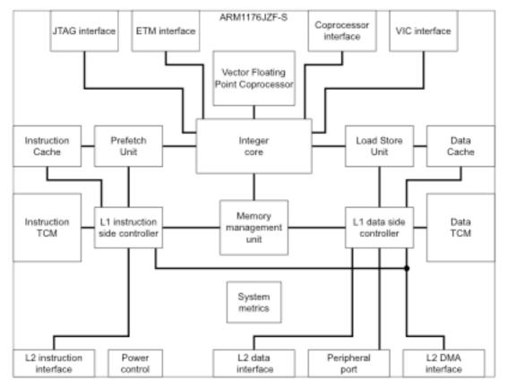
Figure 1-1 ARM1176JZF-S processor block diagram
