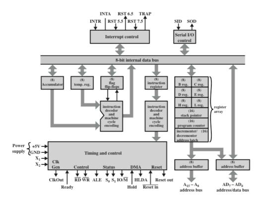
Figure 16.7 Intel 8085 CPU Block Diagram
